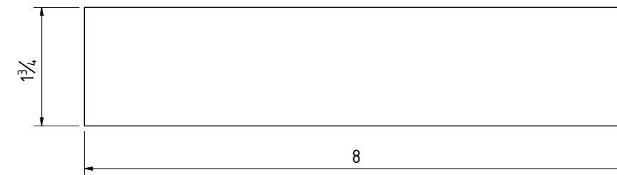
Balcony-P89 | PL 8" x 1.87" x 1/8" MATERIAL: Steel A36 - QTY REQ'D: 4
